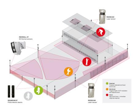
Use Optex detection technology in various indoor and outdoor areas for complete perimeter motion detection
