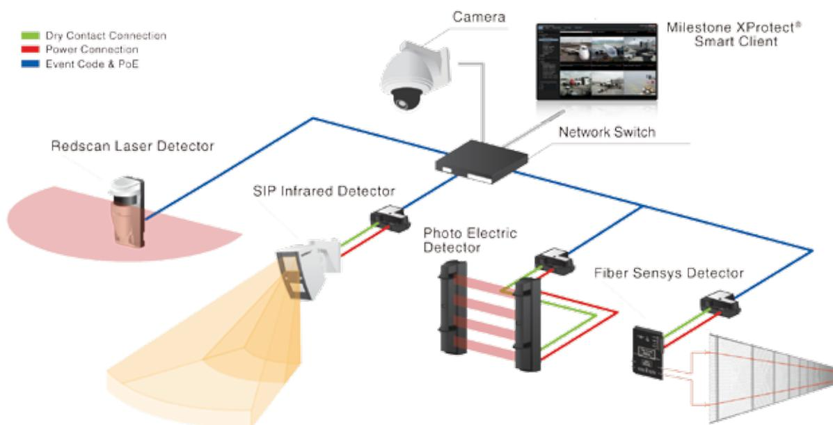
Integrating Optex IP sensors/detectors into XProtect Corporate and XProtect Enterprise video management software (VMS) links data from detectors with video from corresponding cameras. Optex sensors/detectors can be configured to trigger cameras to start recording, allowing surveillance operators to visually verify detections and help reduce the number of false alarms.
