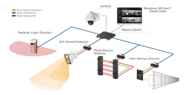
Integrating Optex IP sensors/detectors into XProtect Corporate and XProtect Enterprise video management software (VMS) links data from detectors with video from corresponding cameras. Optex sensors/detectors can be configured to trigger cameras to start recording, allowing surveillance operators to visually verify detections and help reduce the number of false alarms.
