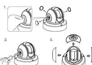
2 Loosen 3 screws and remove the base.
