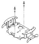
5 Connect safety wire (not provided) with the hole on the mounting plate. (This process is recommended.)
