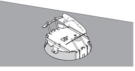
2. Hold the ceiling plate in between the holding bracket and mounting plate.
