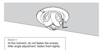
14 Fit front cover, then put lids on the recess mount cover.
