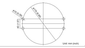
2 Fit the mounting bracket of RLS-2020 on the mounting plate of RLS-RB.
