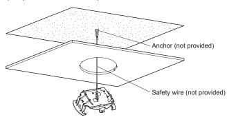
6 Put the mounting plate in the hole, and then slide the holding bracket to hold the ceiling between the mounting plate and the holding bracket as below.
