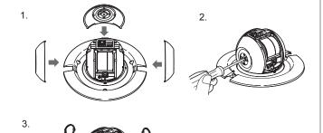
Note>> When using the maintenance port, do not fit the front cover.
